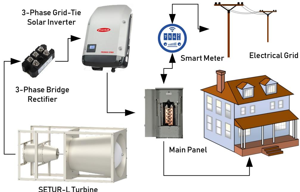
Optionally, the SETUR turbine may be equipped with the HYBRID inverter in support of both on- and off-grid system configurations. This inverter combines a battery charging system, battery inverter, hybrid inverter, controller and system monitoring solution in one device.
